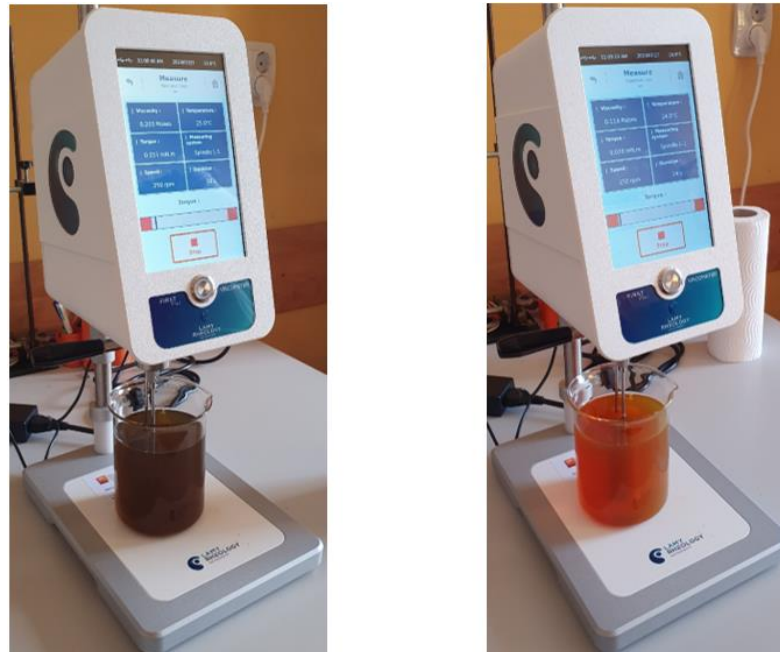
Figure 45: Viscosity measurements of fluids analyzed using DLS technique. On the left is the brake fluid (measured viscosity 0.0202 daP) and on the right is the coolant (measured viscosity 0.0102 daP).
