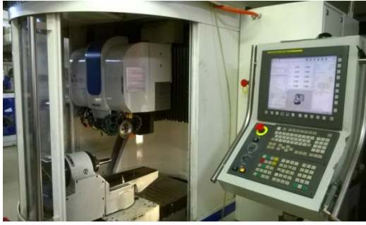
Fig. 6.40. Walter Helitronic Minipower grinding machine (SC COMPA SA)
