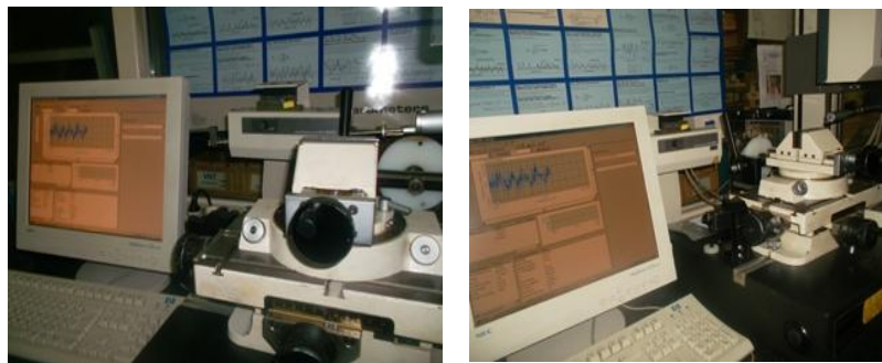
Fig. 6.49. MITUTOYO roughness tester
