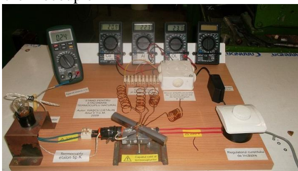
Fig. 6.27. Stall for the calibration of the thermocouple
