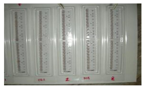
Figure 6.1. Tests API 20 AUX C for the identification of wine yeasts to genus Saccharomyces cerevisiae
