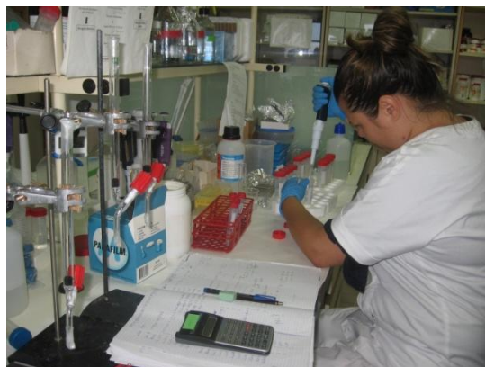
Fig.4.10 Sample preparation for the determination of phosphorus in almond milk ( personal archive )
