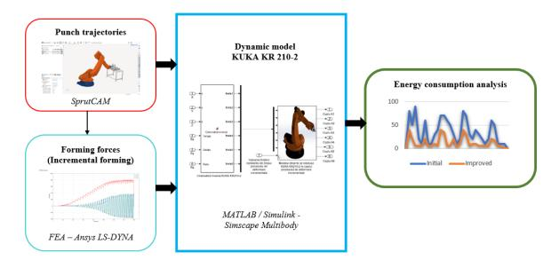
*Fig. I: Block diagram corresponding to the development of the algorithm for establishing energy consumption.*
