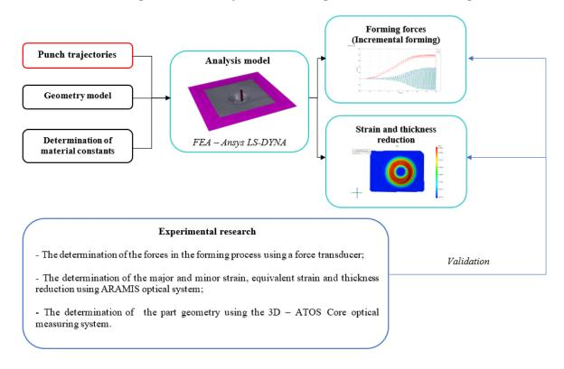
Fig. II: Validation block diagram of the analysis model using FEM.
