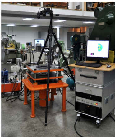
Fig. 17 The experimental installation with the Aramis optical measurement system used for the equibiaxial tensile tests
