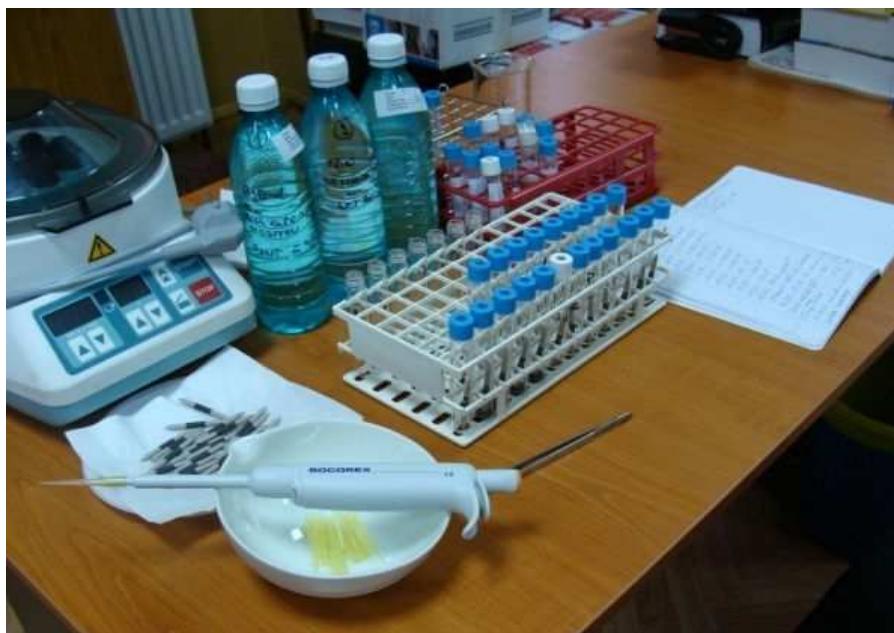
Figure 5.5.5.: Preparation of samples for balancing the system GasBench II (LAFMCA- ICSI Rm Vâlcea)
