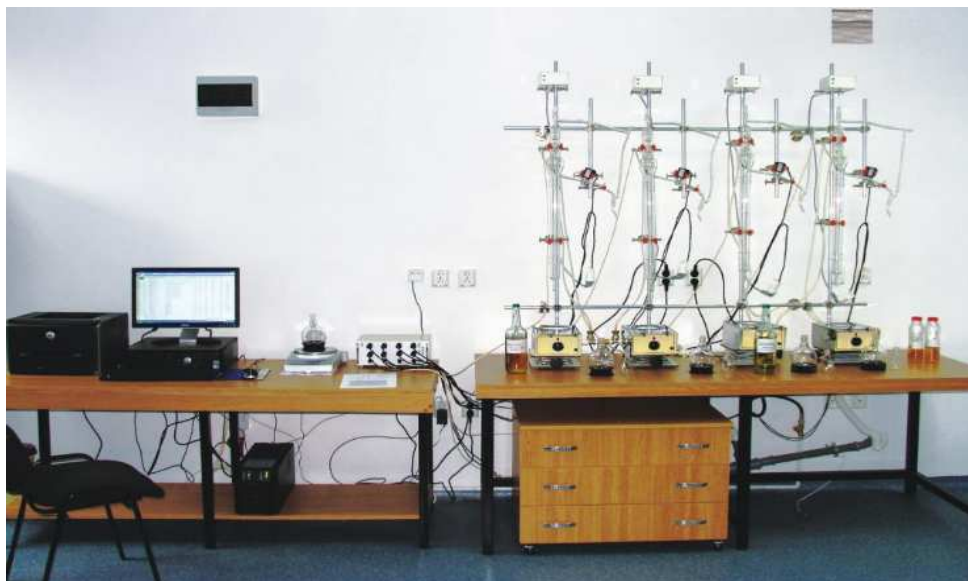
Figure 5.5.4.: System fractional distillation automatically four collars CADIOT –A.D.C.S. (LAFMCA- ICSI Rm Vâlcea)
