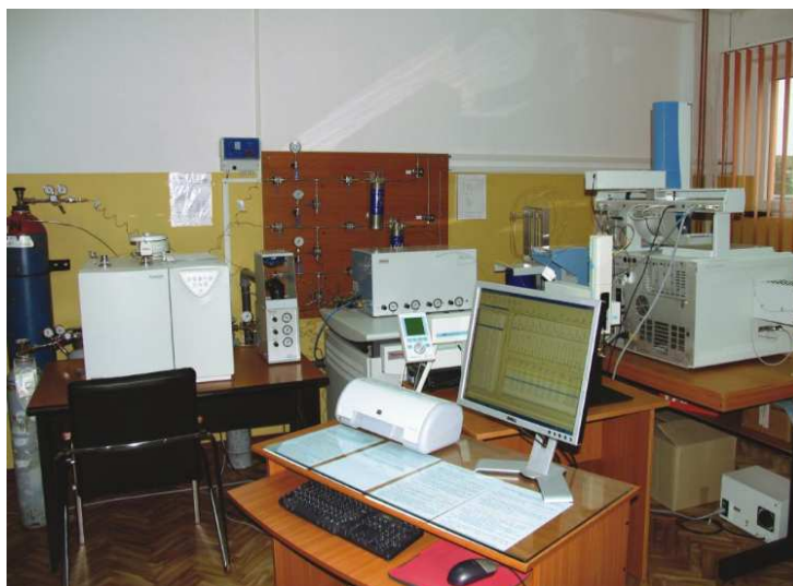
Figure 5.5.1.: Continuous flow mass spectrometer to determine reports of stable isotopes CF-IRMS DELTA V Plus (LAFMCA- ICSI Rm Vâlcea)
