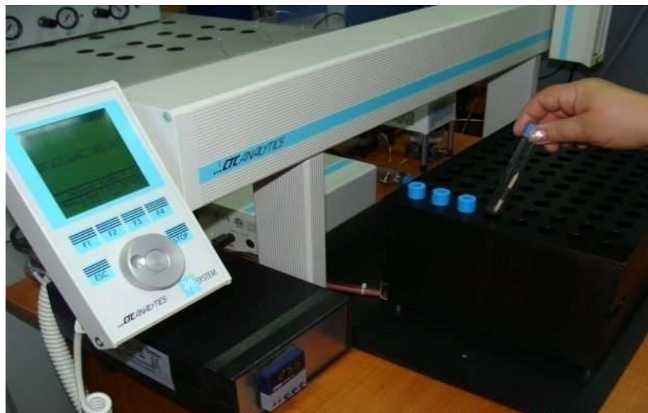
Figure 5.5.6: Introduction the vials with sample in the system of balancing GasBench II (LAFMCA ICSI Rm Vâlcea)
